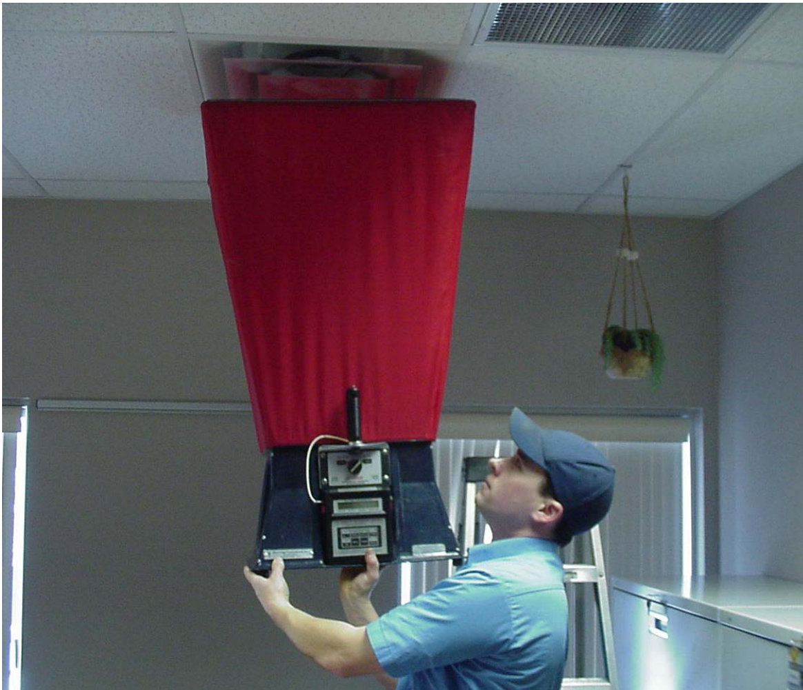
Figure 8-3 Monitoring Air Flow to Balance Pressure within a Building
